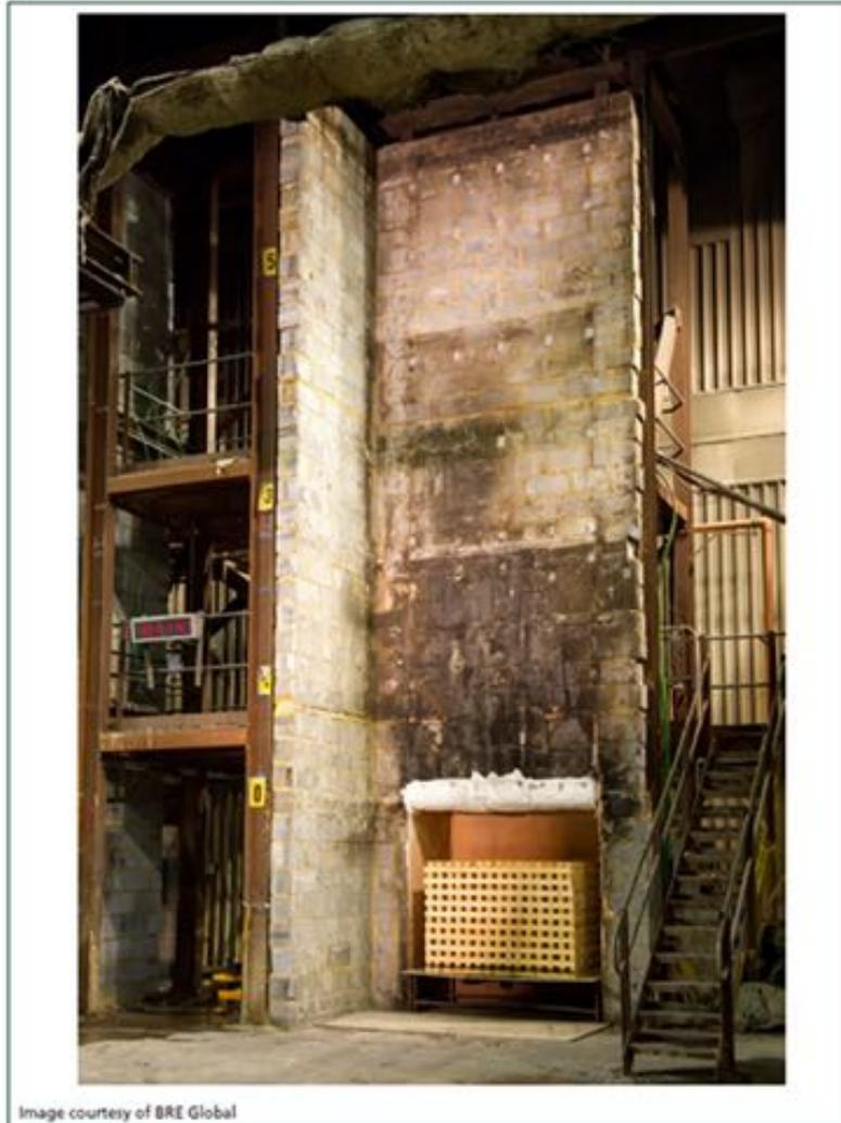
Figure A.10 – B5 8414-1 rig with a timber crib fully alight but no specimen installed, indicating severity of test when there is no contribution from a test specimen
