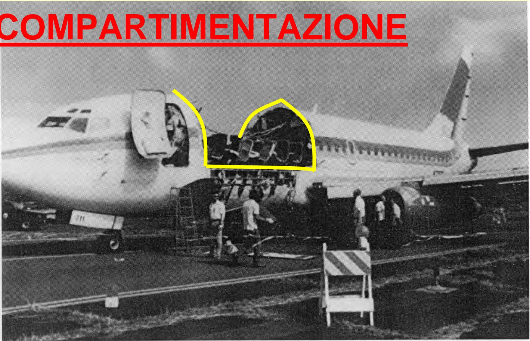
**Figure 1.6.** April 1988 example of service-induced damage that led to explosive decompression and loss of large portion of fuselage skin when small fatigue cracks suddenly linked together. The subsequent fracture was eventually arrested by fuselage frame structure, and the aircraft landed safely (Photograph courtesy of the National Transportation Safety Board.)
