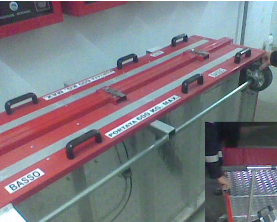
Trolley for transporting rescue equipment on the line
