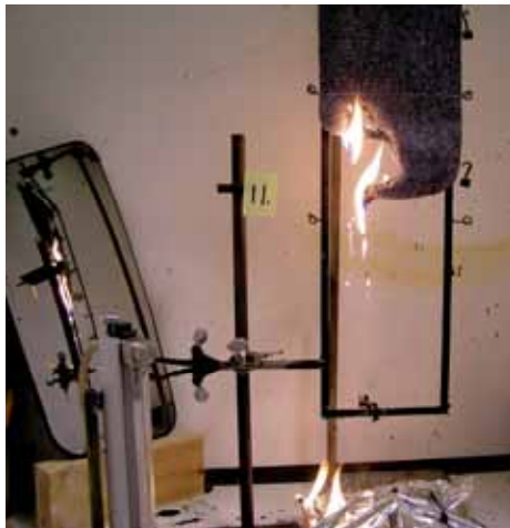
ISO 6941 (ECE Reg No 118 annex 8), vertical burning rate
