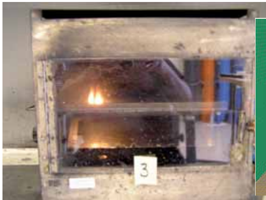
ISO 6941 (ECE Reg No 118 annex 8), vertical burning rate
