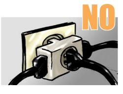
(iron, heater etc.) is strongly discouraged. Do not exceed the capacity of the wiring system: over-
