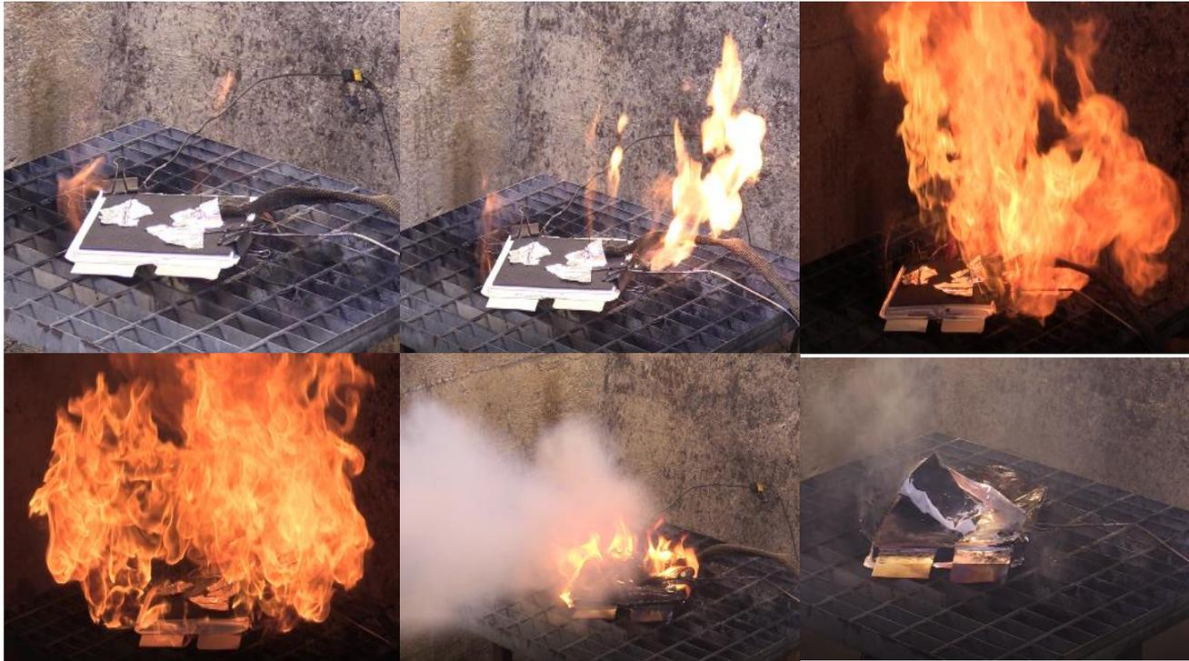
K40-P-CO<sub>2</sub> test: (a) ignition, 0s; (b) venting, 10s; (c) swelling, 15s; (d) catastrophic rupture, 60s; (e) extinction, 65s; (f) post extinction, 75s.
