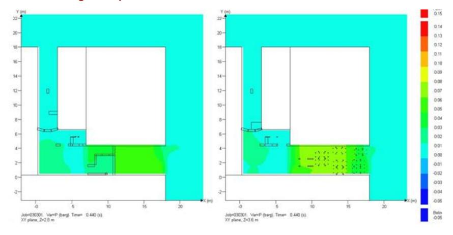
Comparison between the maps of pressure under (2.8 m) and over (3.6 m) the mezzanine floor, 0.440 s after the ignition of 5 L of fuel
