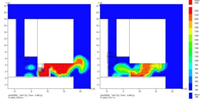
Maps of temperature at 0.6 m of height on the ground floor (left) and at 0.45 m of height on the mezzanine floor (right), 0.494 s after the ignition
