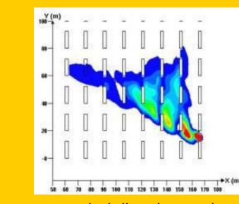
Gas dispersion (same release rate, gas type, wind direction, etc)
