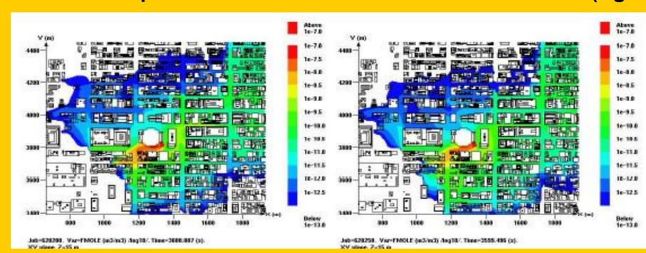
■ Tracer gas calculations (right) compared with "experimental" data (left) from real releases
